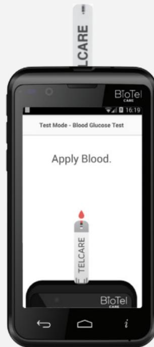
1 Power on and insert a new test strip until it is fully seated and Apply Blood appears.
