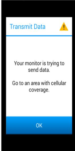
Cannot find a cellular tower. Triggered when an event is pending for longer than 30 minutes. Move to an area with cellular service.
