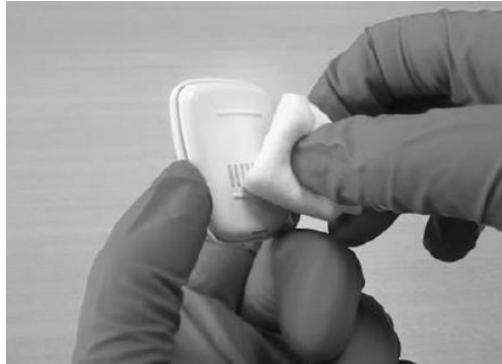
*Figure 22-1 Cleaning the Sensor*
