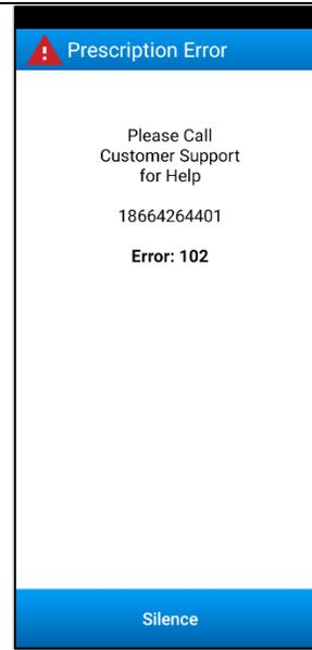
If the Monitor does not receive an enrollment after a configured amount of time, and *Warning 102* has already displayed, then *Error 102* will display. The error cannot be dismissed. Contact Customer Support 866-426-4401.
