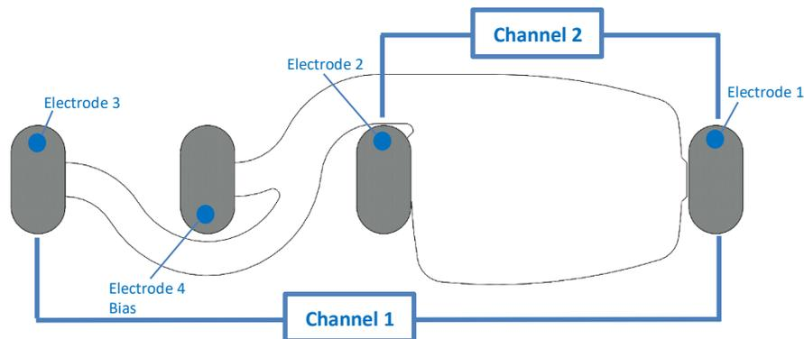
The Patch has four electrodes. Channel 1 is formed by Electrode 1 and 3. Channel 2 is formed by Electrode 1 and 2. Electrode 4 corresponds to the bias electrode.
