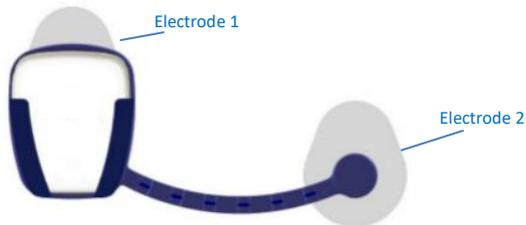
The Flex Adapter utilizes two electrodes. Channels 1 and 2 are formed by Electrodes 1 and 2. Channel 1 and Channel 2 are connected in parallel.
