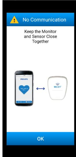
No communication between Sensor and Monitor triggered when Monitor can no longer detect Sensor. Keep the Monitor and Sensor close together.
