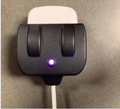
Figure 22.2-1 Pulsing Pink LED indicates purging device
