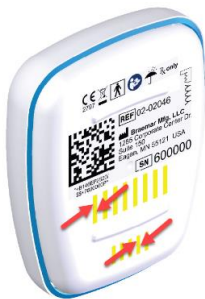
a. Crevices at the edges of electrical contacts example
