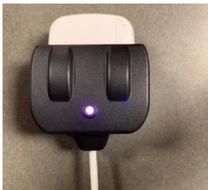
Figure 22.2-1 Pulsing Pink LED indicates purging device
