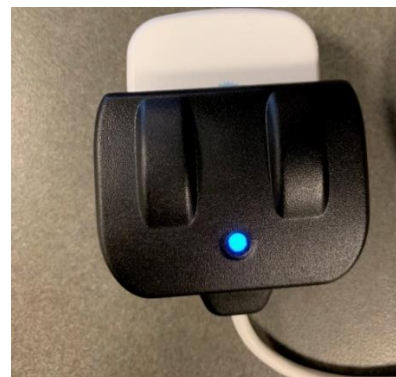
Figure 22.2-2 Pulsing Blue LED indicates charging. Solid Blue indicates charge complete
